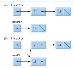
**Fig. 19.6** Operation insertAtFront represented graphically.
