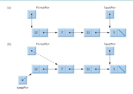
**Fig. 19.8** Operation removeFromFront represented graphically.
