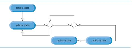
**Fig. 5.25** Activity diagram with illegal syntax.
