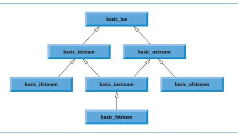
**Fig. 14.2** Portion of stream I/O template hierarchy.
