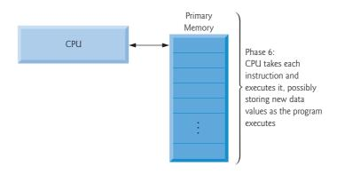
**Fig. 1.11** Typical C++ development environment—execution phase.
