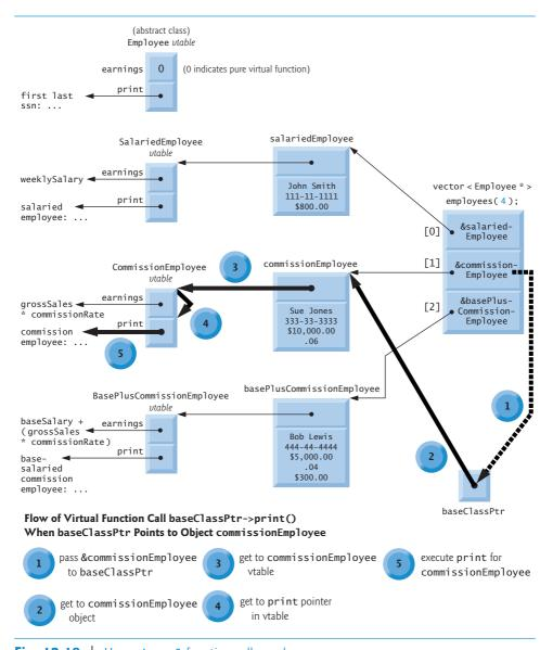
**Fig. 12.18** How virtual function calls work.
