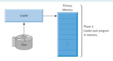
**Fig. 1.10** Typical C++ development environment—loading phase.
