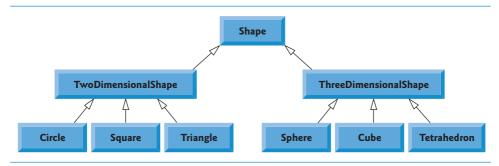
**Fig. 11.3** Inheritance hierarchy for Shapes.
