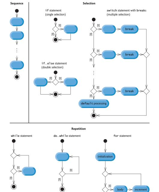
**Fig. 5.20** | C++'s single-entry/single-exit sequence, selection and repetition statements.
