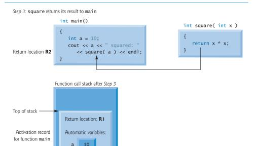
**Fig. 6.17** Function call stack after function square returns to main.
