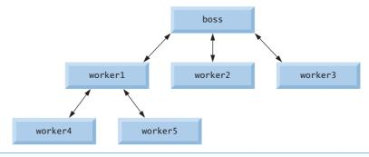
**Fig. 6.1** Hierarchical boss function/worker function relationship.
