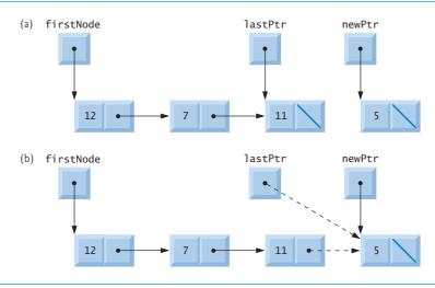
**Fig. 19.7** Operation insertAtBack represented graphically.
