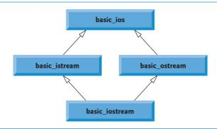
**Fig. 13.1** Stream-I/O template hierarchy portion.
