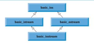
Fig. 23.12 | Multiple inheritance to form class basic\_iostream.
