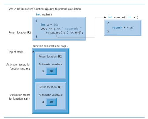
**Fig. 6.16** Function call stack after main invokes square to perform the calculation.
