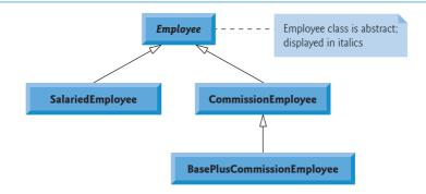
**Fig. 12.7** Employee hierarchy UML class diagram.
